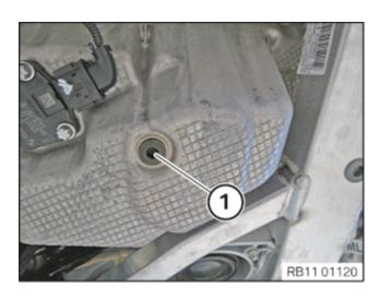
Open oil drain plug (1) on oil sump.
