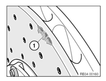
friction surfaces may make it necessary to change the brake discs.
