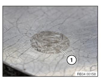
As the brake disc is used, the surface structure of the wear indicators (1) changes. The change in this surface structure provides an indication of the wear state of the brake disc.
