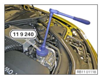
Secure oil filter cover with special tool 11 9 240.
