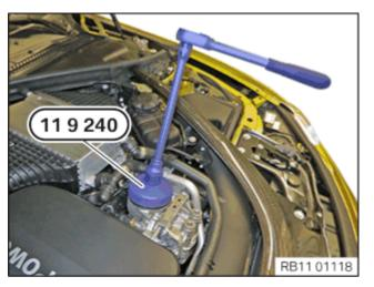
Release oil filter cover with special tool 11 9 240.
