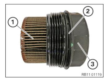
Remove the filter element (1) from the housing (3) and re-insert.
